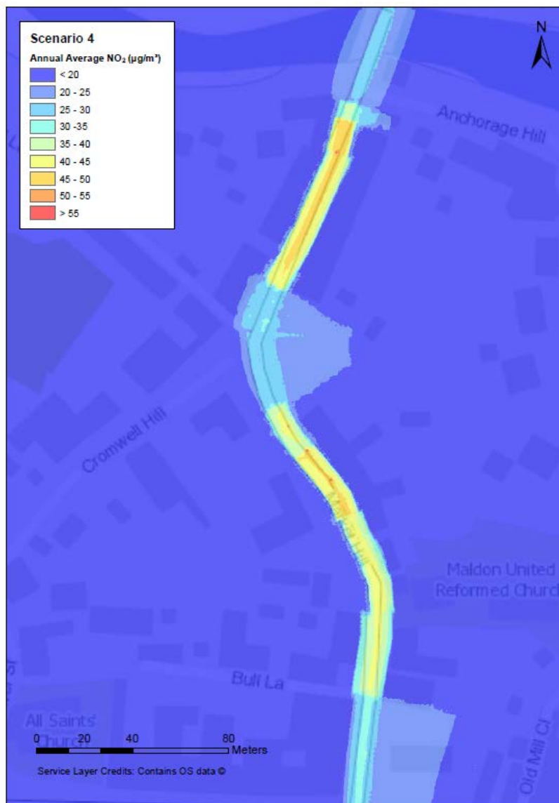
Figure 4.1 - Modelled Annual Average NO 2 Concentrations for a Class B Clean Air Zone
